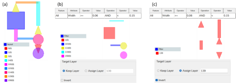
Figure 8. a) Layout with several layers. Filter to select features between 60 and 150 nm where b) keeps their layering, and c) assigns a new layer (139) and applies a NOT operation to the filter instruction (Invert).
